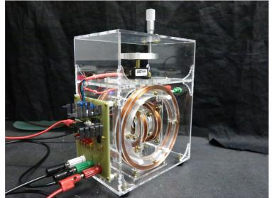
The apparatus is smaller than a breadbox, connects to a standard USB port for data collection and instrument control, and uses no special lab equipment or dedicated computer hardware. It is controlled by a Teensy<sup>™</sup> microcontroller which synthesizes the drive signal and tracks position and velocity of the rotor. (Click on photo for a higher resolution view.)
