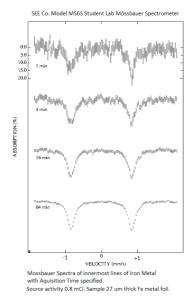
Mössbauer spectra showing lines 3 and 4 of the sextet of a 27 um thick natural Iron foil at room temperature. Data acquisitions times are noted. The Co-57 source activity was 0.8 mCi. The sample had diameter 18 mm and was 35 mm from the source.
